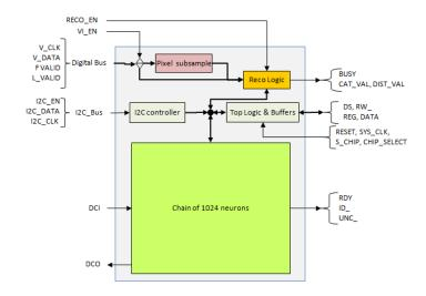
A single CM1K matching a pattern of 256 bytes against 1024 models delivers the equivalent of 192 GiGaOps per second.
