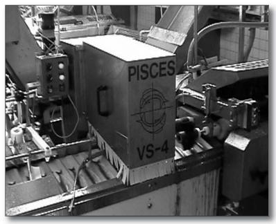
Figure 6. The CogniSight System Installed on the Filleting Line.
