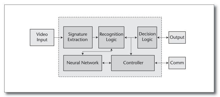
Figure 8. CogniSight Image-Recognition Engine Architecture.
