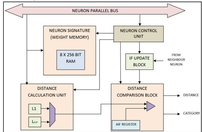
Figure 4. Simplified Architecture of a Neuron
