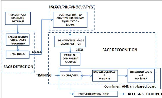
Figure 1. Data-flow diagram of ANN board based Face recognition system
