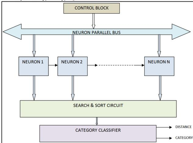
Figure 3. Functional block diagram of the Neural Network chip
