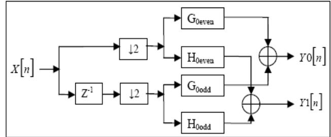
Figure 2. Poly Phase decomposition of Input Sample
