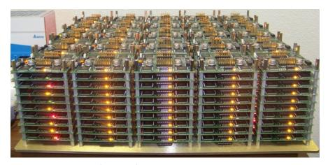
In 2012, Guy Paillet and Anne Menendez have built at their Petaluma office (California) a BAB of 1 million neurons (beside) composed of 25 columns of 10 stackable NeuroStack boards with each four CM1K chip, totaling 4096 neurons per board. The CM1K chip is a neuronal component which has 1,024 neurons corresponding to 256 inputs and 16,392 outputs with
